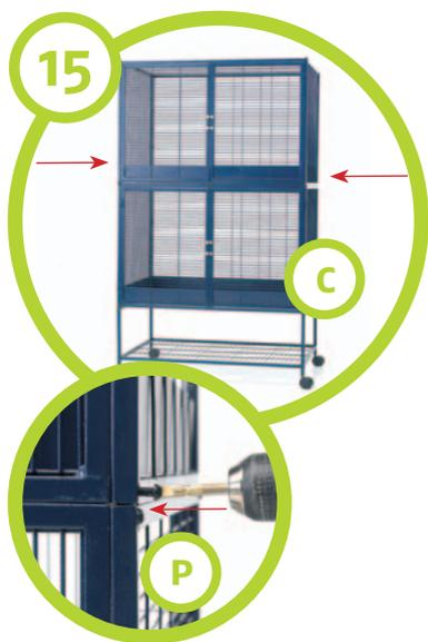
Install the remaining side panels (C). Make sure the pins of the grid are firmly secured in the holes of the side panels. Attach the side panels to the front and back panels with screws (P). Tighten all the screws where necessary.
