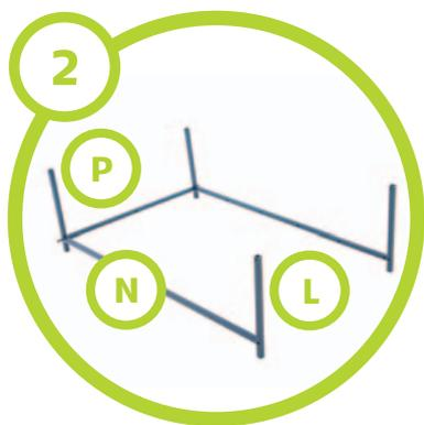
Attach the second H-shape tube (N) to the tube with hole (L) with a screw (P) and once again do not tighten. Make sure that the holes of the tube are facing inwards.
